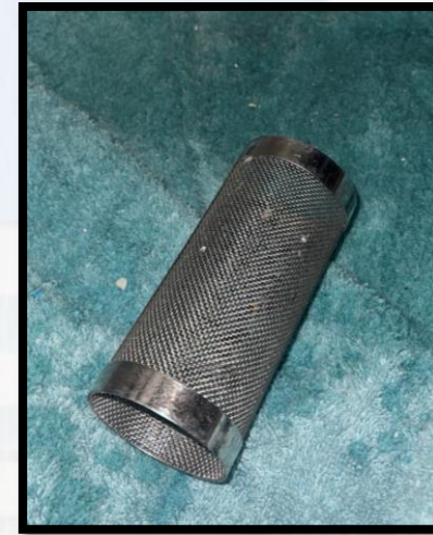
Clean strainer during routine maintenance
