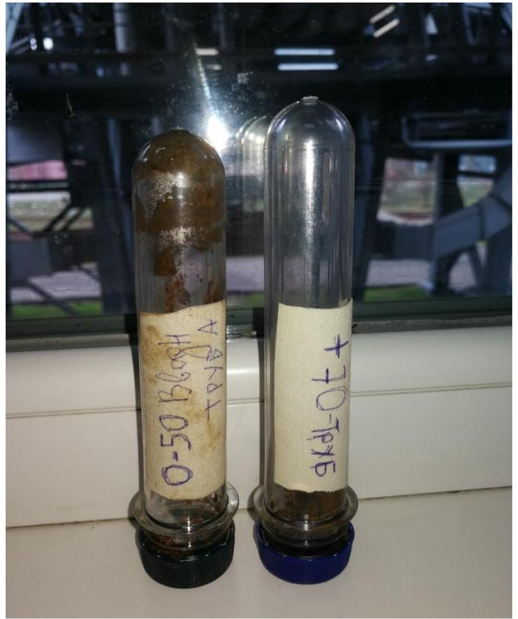
*Sampling deposits from the inner surface of the wall of the heat transfer tube*
