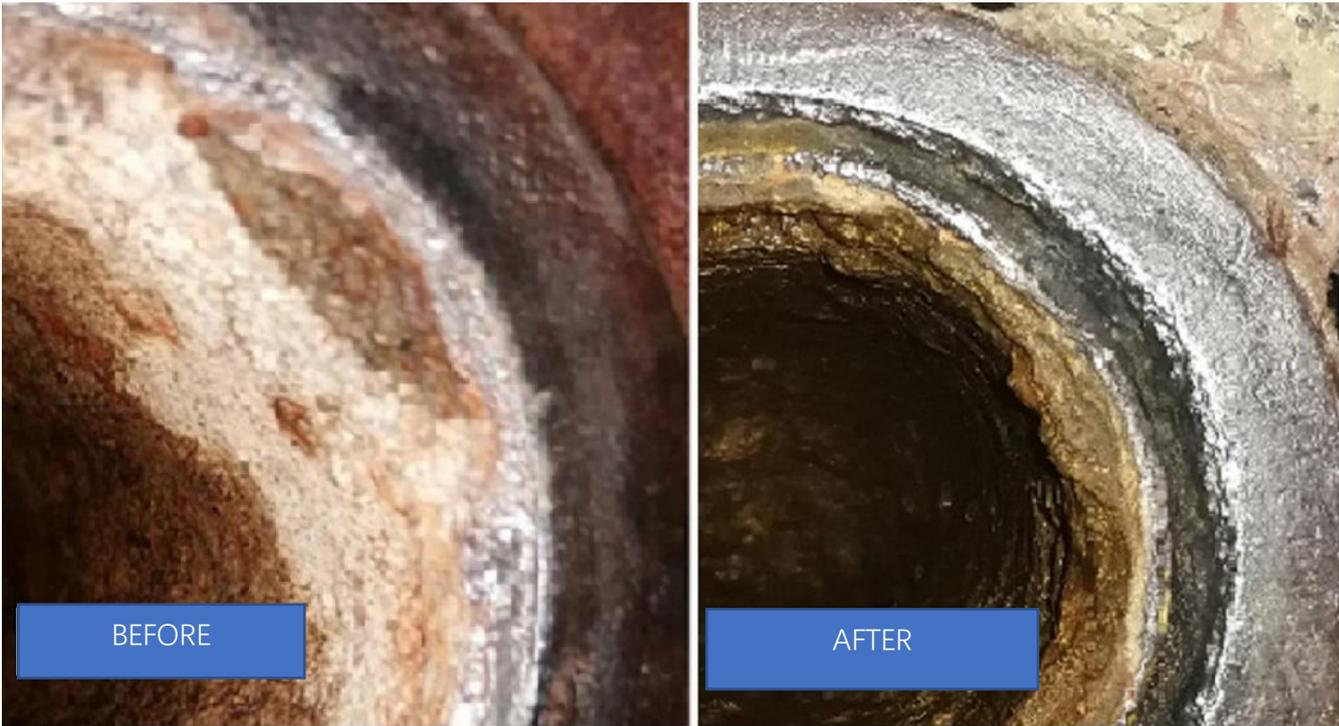
*Comparison of the state of the inner surface of the the industrial water supplying pipe at the beginning and at the end of the test installation*
