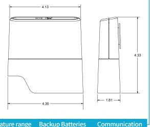
DimensionsWeightVoltageRadio frequencyTemperature rangeBackup BatteriesCommunication4.33"/4.13"/1.81"5.110Z110V-240V915MHz-4° to 122° F2 x AAWIFI/SIM/ETHERNET
